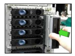
4. Secure the drive cage with a screw.
